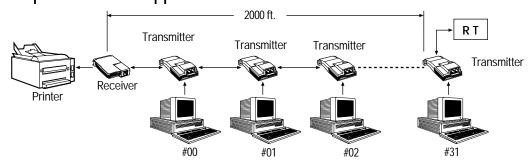
Up to 32 PCs can share the same printer at speeds up to 250 kbps and distances up to 2000 feet (610 m).
