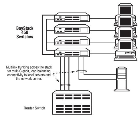
The BayStack 450 Switches can help you get 10/100/1000 switching in the wiring closet, featuring fail-safe stackability and multilink trunking for redundant connections to local servers and the network center.
