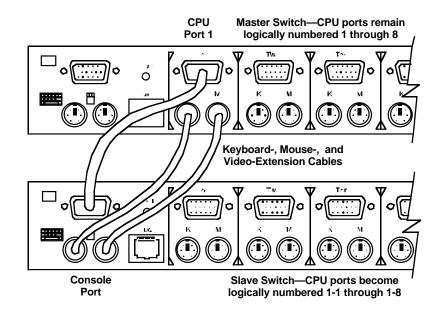
When your system is fully installed, you can use up to four monitors, keyboards, and mice to control as many as 64 computers. And you don't have to toss your existing Compaq or HP switches—just plug them right into the system, as either masters or slaves.
