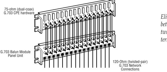
Eliminate mismatches between coax and twisted-pair G.703 terminations.
