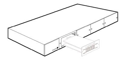
Each chassis slot functions as a MAU, an RI/RO unit, or a Repeater—just add the appropriate module!
