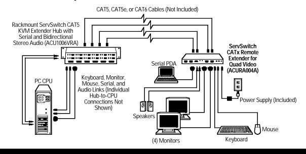
interconnect ports. The first port carries primary video and data signals, and the other ports carry additional video signals. What's more, the ServSwitch Brand CATx Remote Extenders for Quad Video also feature surge protection on each RJ-45 port.
