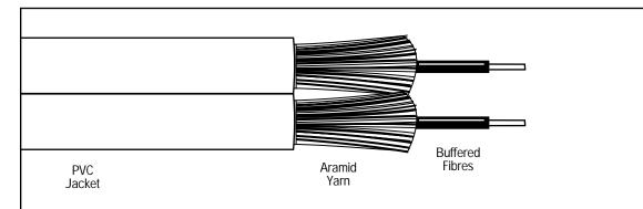
This general-use 62.5- and 50-micron breakout cable is designed for long runs.
