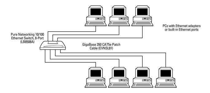
Use 10/100 Ethernet Switches as hubs to build a small network or to add more PCs to your existing network.
