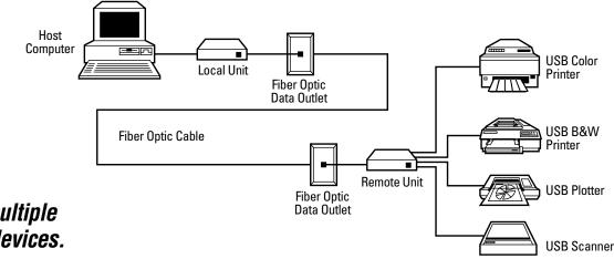
Connect multiple colocated devices.
